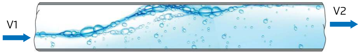
Fig. 31 Air pockets inside the pipe
