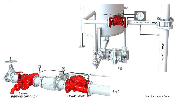
In Fig. 2 the 400Y-C-06 is installed to prevent excessive flow, protecting the dosing pump from overflow damage often experienced during pump start up and during initial system pipe filling.
