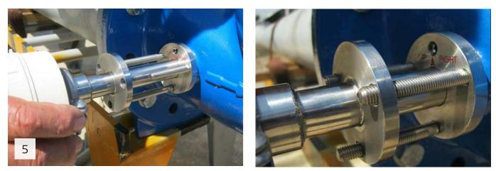
Use the table below to select the correct three 'Short' or 'Long' stud bolt according to the valve DN size. Use the supplied 6mm wrench to screw-in the painted green side of the stud bolt till the stud bolts are locked against their thread end
