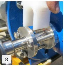
Select the correct spacer combination according to valve's size using the table below
