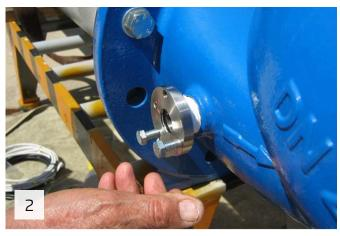
Screw the sealing disk into the 1" BSPT port; use two regular screws to lock the disk temporally in the up-right position as indicated on the disk. Tighten the disk gently
