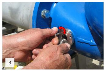
Remove the temporary screws from the disk
