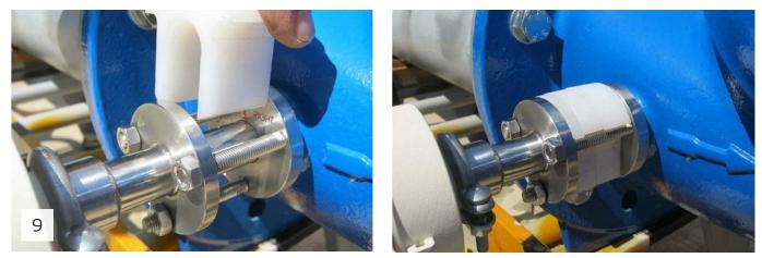
Tighten the nuts but make sure not to apply excessive torque, it may damage the plastic spacer
