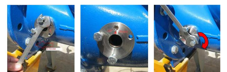
**Important:** do not tie the sealing disk till the very end of its tread; only position it in the up-right position \* If overrides, unscrew it backwards to the correct position **Note:** Do not apply excessive torque, tighten gently!
