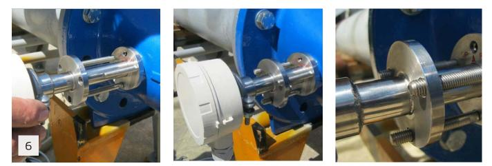
Carefully insert the sensor into the disk, make sure not to damage the O-ring **Note:** that the sensor can be inserted in one position only
