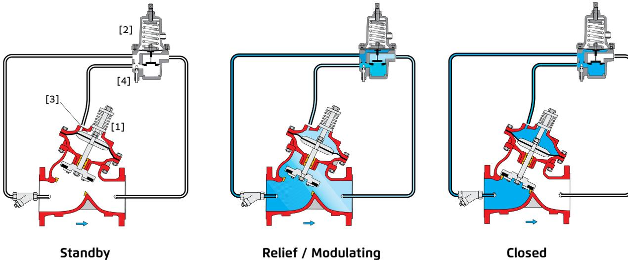
**Standby:** The BERMAD 730-48 is a Normally Open valve with an external lifting spring [1] keeping the valve in a fully open position as default when the system piping is depressurized, as might be before a pump start-up. When the pump starts the initial pressure surge and excess air will be expelled from the system through the valve.
