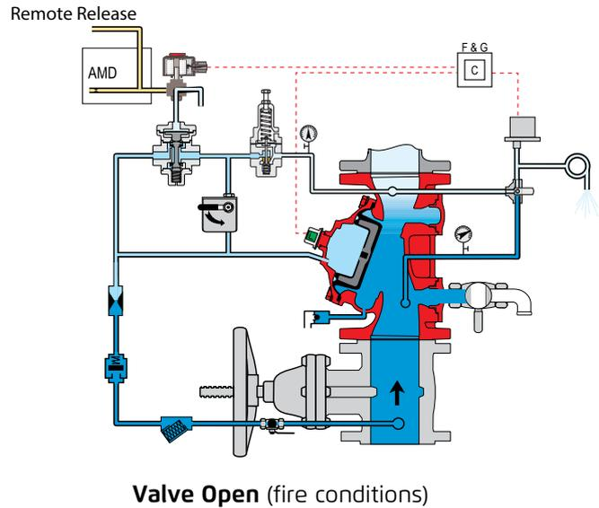
The BERMAD model 400Y-6DC is held closed by water pressure in the control chamber [1]. Upon release of pressure from the control chamber, the valve opens.
